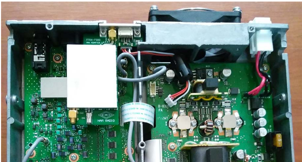
Insertion of PTRX-7300 Panadapter Module
